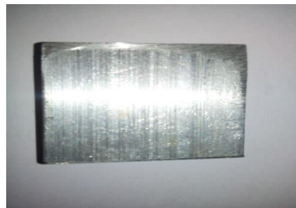
Fig 1. This figure shows the Microchannel substrate before WEDM
