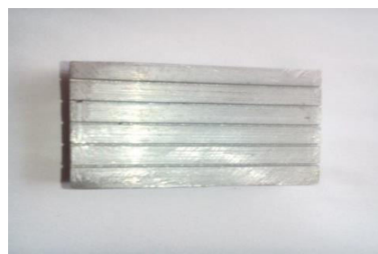
Fig 2. This figure shows Microchannel substrate after WEDM.
