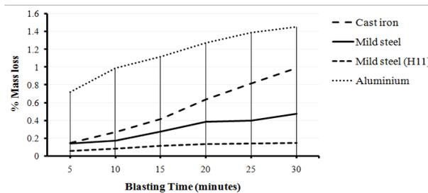
**Fig 3: Effects of Blasting Time on % of Mass Loss**
